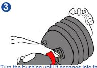
Turn the bushing until it engages into the guard.
