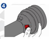
Push Easy Lock clip into position. The bushing and guard are now secured.
