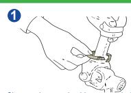
Clean and grease bushing groove before the bushing is placed in the groove. Grease any remaining bushings in guard.
