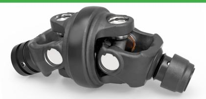
The constant velocity universal joint (CV) allows smooth machine operation through a broad range of motion. These joints allow the machine to be designed with the input shaft in the best operating position and yet allow the operator to maneuver as needed. The CV delivers constant power by self-canceling torque and speed fluctuations typically found in single cardan-type universal joints.
